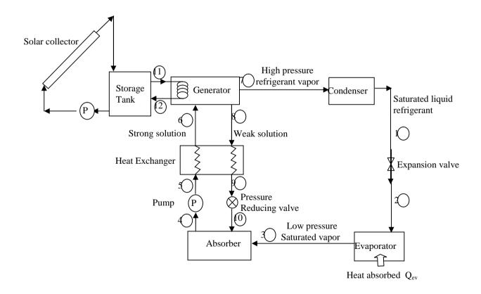
Figure (1). Solar powered air conditioning system.
