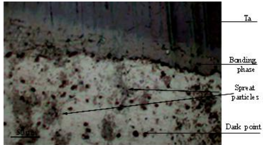
Figure (2) . (Ta – to - Ta ) assembly brazed by Ag 4 Ti filler metal .
