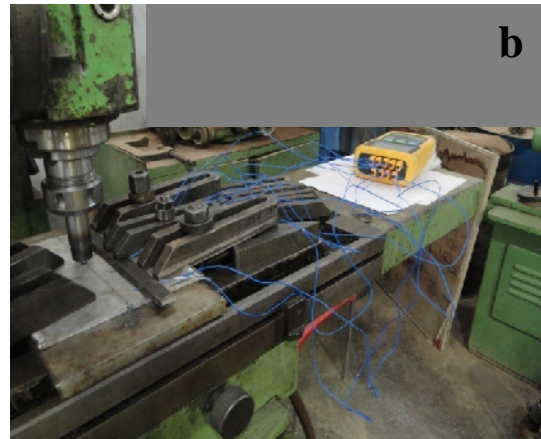
Figure(2-2).Shows (a) thermocouple reader connect with 9- K type thermocouples,(b) thermocouples distributes along the workpiece surface, and (C) The tool move with rotational speed 1400 rpm and travel speed 110 mm / min.
