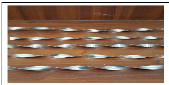
Fig .2 Typical twisted tape
