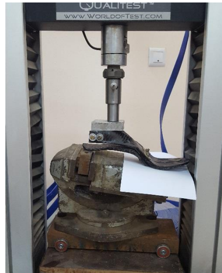
Figure (4) the new prosthesis under plantarflexion test.
