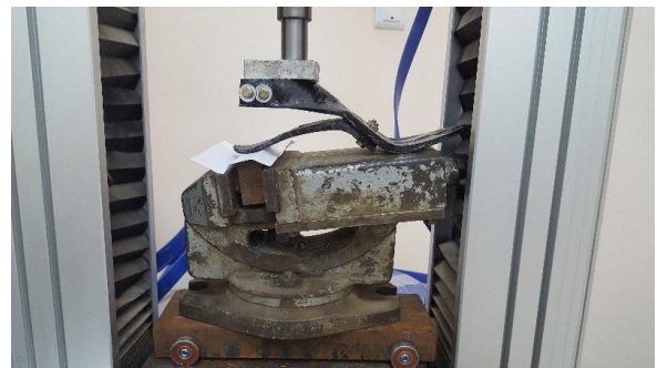
Figure (2) the new ankle-foot prosthesis under dorsiflexion test.
