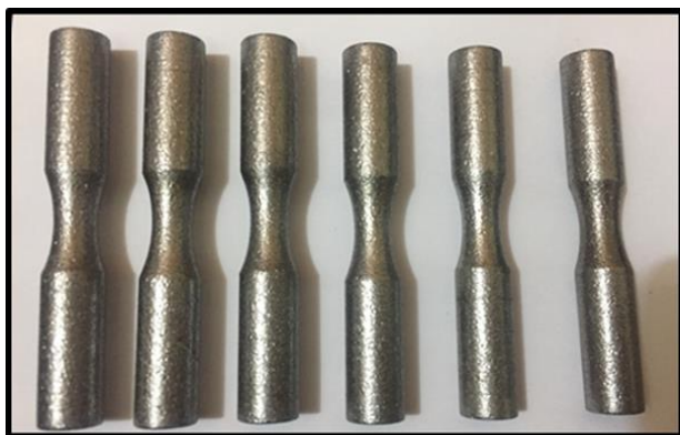
Fig.(4) the surface of specimens after shot peening at 20min.
