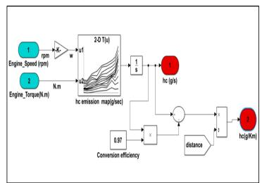
Figure (7) Calculation Of HC Emission
