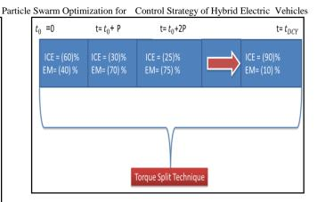
Figure (4) Torque Split Technique
