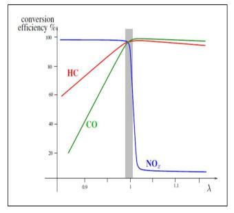
Figure (6) Catalytic Converter Efficiency (Leroy et al., 2007)
