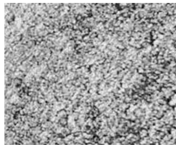
(j) Al 7075 laser heat treatment (depth =100 μm),1000 mJ
