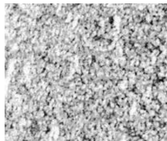
(k) Al 7075 laser heat treatment (depth =300 μm),1000 mJ
