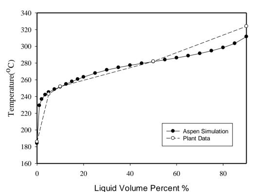
Figure 8: Simulated and plant data ASTM D86 curves of LGO.
