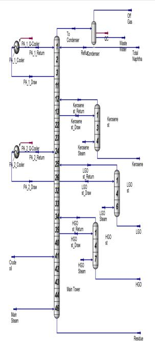
Figure 3: Refinery process flow diagram simulated in Aspen Hysys.
