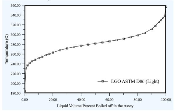
Figure 5: Simulated ASTM D86 curves of LGO.
