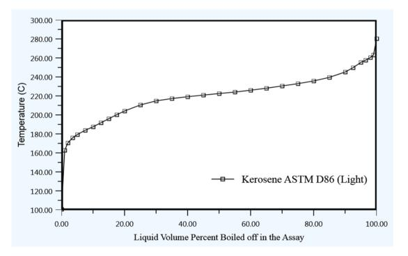
Figure 4: Simulated ASTM D86 curves of Kerosene.
