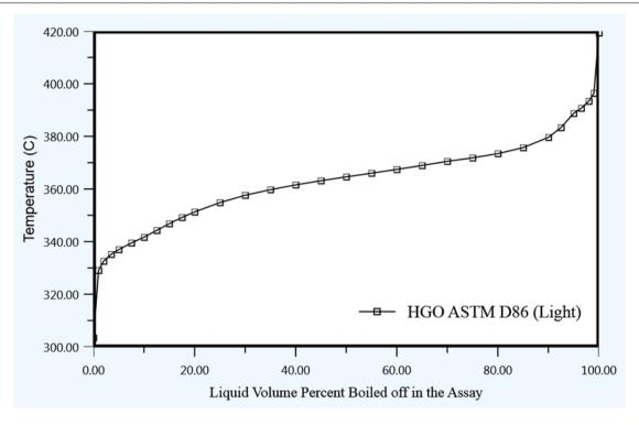
Figure 6: Simulated ASTM D86 curves of HGO.
