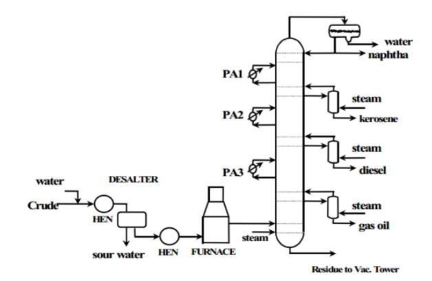
Figure 1: Typical Crude Distillation Unit and Associated Unit Operations.
