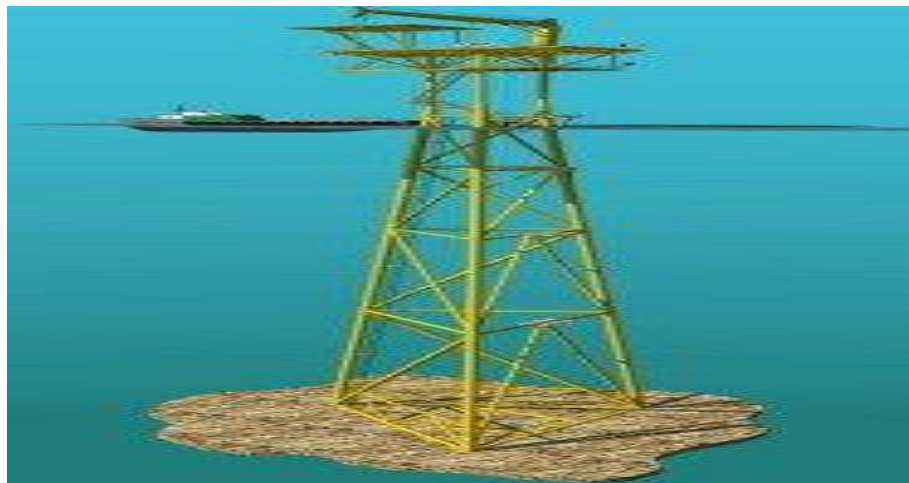
Fig(2): Fixed part of mooring platform
