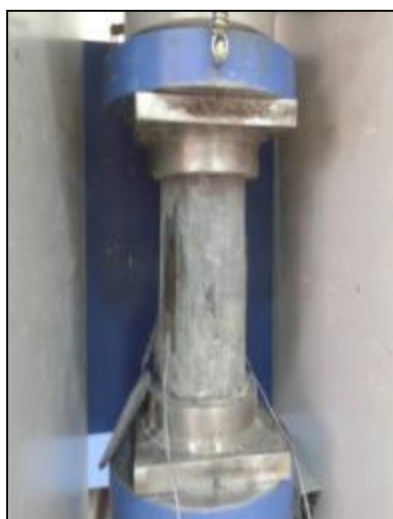
a) 2 strain gauges for tested cylinder
