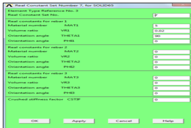
Figure (10). Input data of steel fiber modeling , One-way ,Vertical distribution
