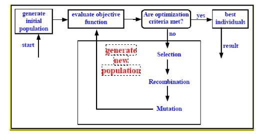
Fig.(1) Structure of genetic algorithm [5].
