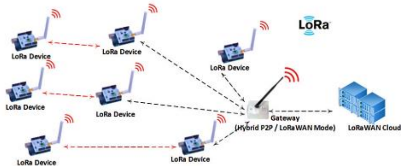
Figure 8: multi hop network in LoRa technology (Misbahuddin et al., 2019)
