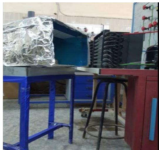
Fig.4: face of the evaporative cooling unit
