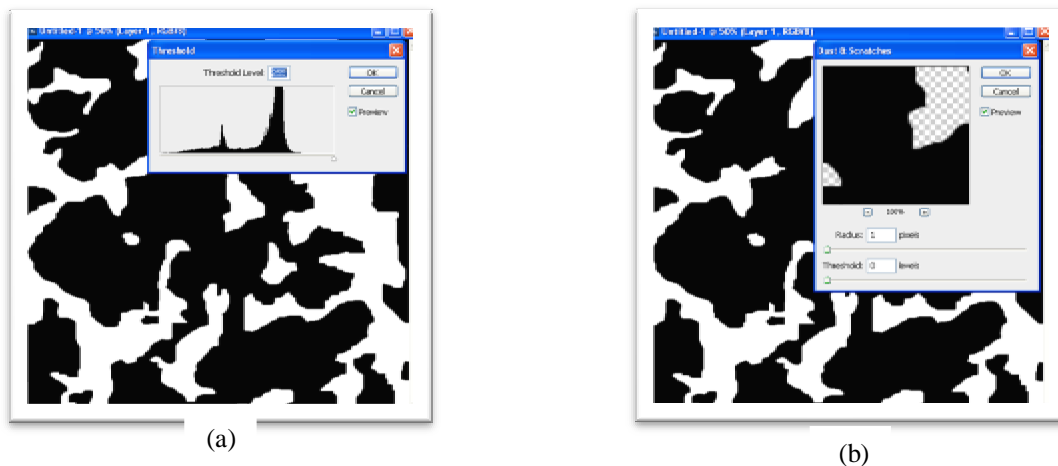
Figure (6). Threshold stage, (a) Threshold step, (b) Dust and scratches step.
