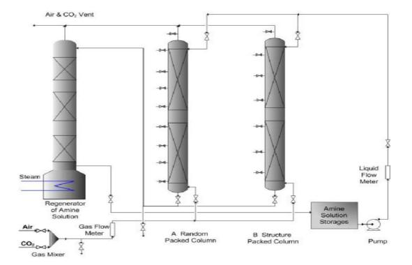
Figure (3). Experimental apparatus for CO<sub>2</sub> absorption.
