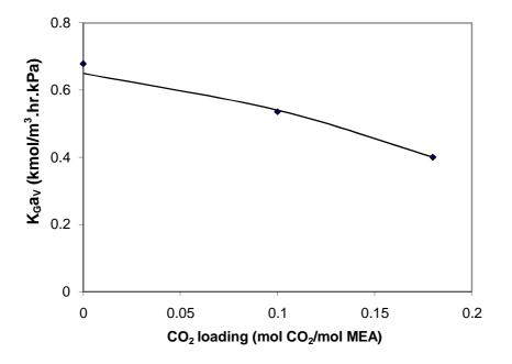
Figure (7). Effect of CO<sub>2</sub> loading of lean solution on overall mass transfer coefficient for CO<sub>2</sub>-MEA system (gas flow rate 9 mol/m<sup>2</sup>.s, liquid flow rate 7.69 m<sup>3</sup>/m<sup>2</sup>.hr, solution concentration 3 kmol/m<sup>3</sup>, CO<sub>2</sub> feed 15%).
