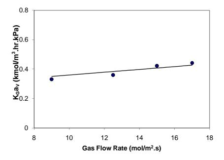
Figure (5). Effect of gas flow rate on overall mass transfer coefficient for  $CO_2$ -MEA system (liquid flow rate 7.69 m<sup>3</sup>/m<sup>2</sup>.hr, solution concentration 3 kmol/m<sup>3</sup>,  $CO_2$  feed 20%,  $CO_2$  loading of lean solution 0.2 mol/mol).
