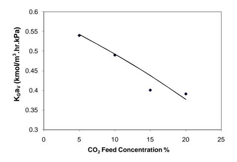
Figure (8). Effect of feed CO2 concentration on overall mass transfer coefficient for CO2-MEA system (gas flow rate 9 mol/m2.s, solution concentration 3 kmol/m3, , liquid flow rate 7.69 m3/m2.hr, CO2 loading of lean solution 0.18 mol/mol).
