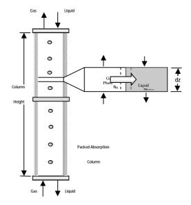
Figure (1) Schematic diagram of a packed column.
