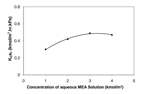
Figure (6). Effect of solution concentration on overall mass transfer coefficient for  $CO_2$ -MEA system (gas flow rate 9 mol/m<sup>2</sup>.s, liquid flow rate 7.69 m<sup>3</sup>/m<sup>2</sup>.hr,  $CO_2$  feed 10%,  $CO_2$  loading of lean solution 0.18 mol/mol).
