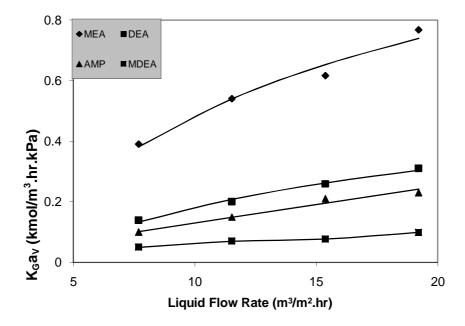
Figure (9). Effect of liquid flow rate on overall mass transfer coefficient for CO2-MEA system (gas flow rate 9 mol/m2.s, solution concentration 3 kmol/m3, CO2 feed 20%, CO2 loading of lean solution 0.18 mol/mol ).
