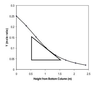
Figure (2) .Determining  $dY_A/dZ$  from the CO<sub>2</sub> mole ratio concentration profile.
