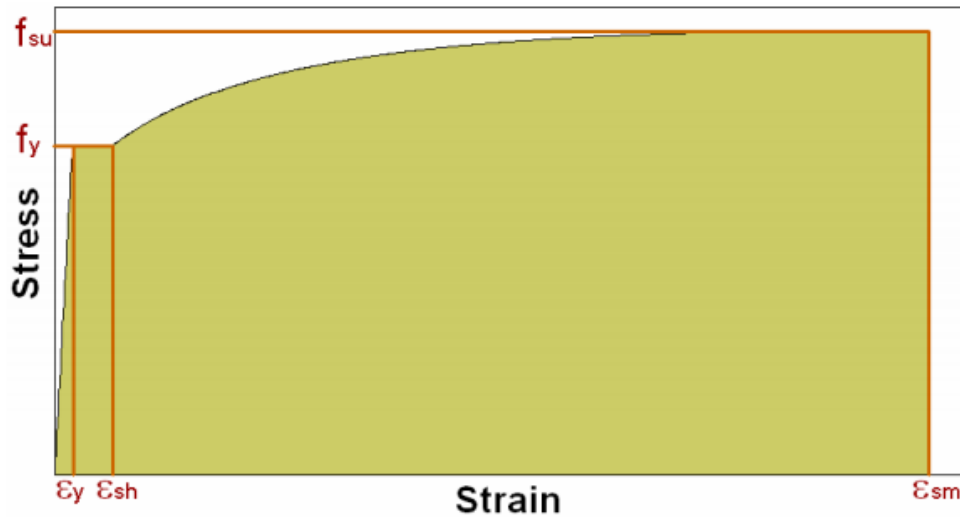
Fig.2 King et al. constitutive model for the reinforcing steel
