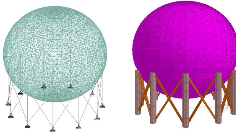
Fig.(6):Finite Element 3D Model Of LPG Spherical Tank
