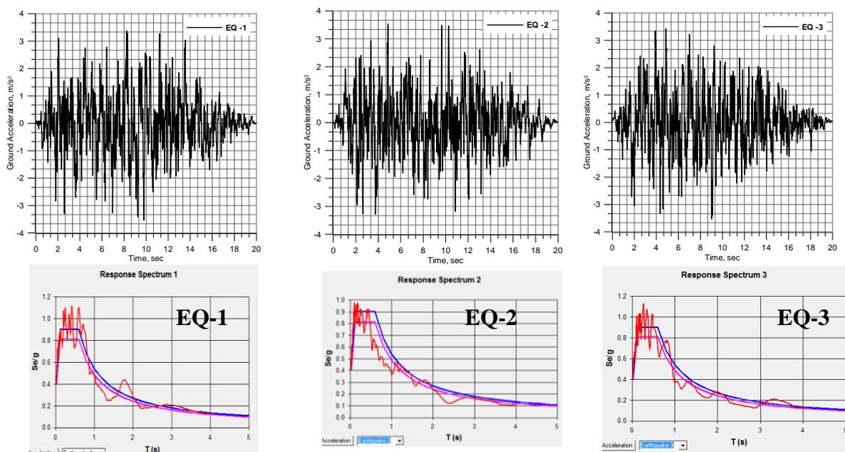
**Fig.(5):** Acceleration-Time Histories of Artificial Earthquakes and Its Spectra
