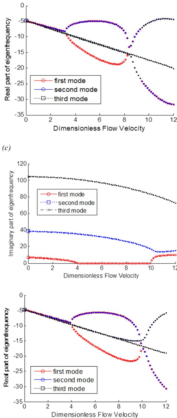
**Fig. 3:** Lowest three modes of cantilever FGM pipe lying on visco-elastic foundation against fluid velocity ( $u$ ) ( $K_m = 50, K_s = 10, C_d = 10$ ) (a) exponent  $k=0$ , (b) exponent  $k=1$ , (c) exponent  $k=10$ .
