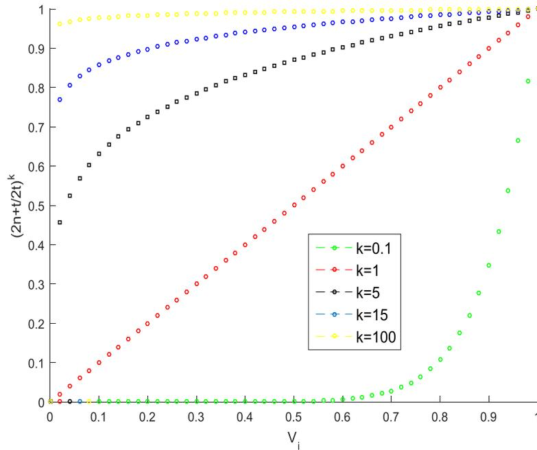
Fig. 2: Volume fraction variations along the thickness of pipe for different values of power gradient index (k).
