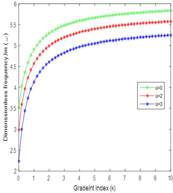
**Fig. 5:** Effect of power law exponent (k) on imaginary natural Frequency with different flow velocity (u) ( $K_m = 50$ ,  $K_s = 10$ ,  $C_d = 10$ ) for (C-F) boundary condition.
