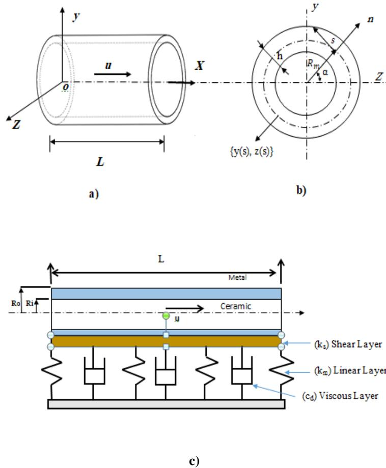
**Fig. 1:** (a) Side view of FGM pipe conveying fluid, (b) cross-section and coordinate system ( $n - s$ ), and (c) Geometry of FGM pipe and visco-elastic foundation.
