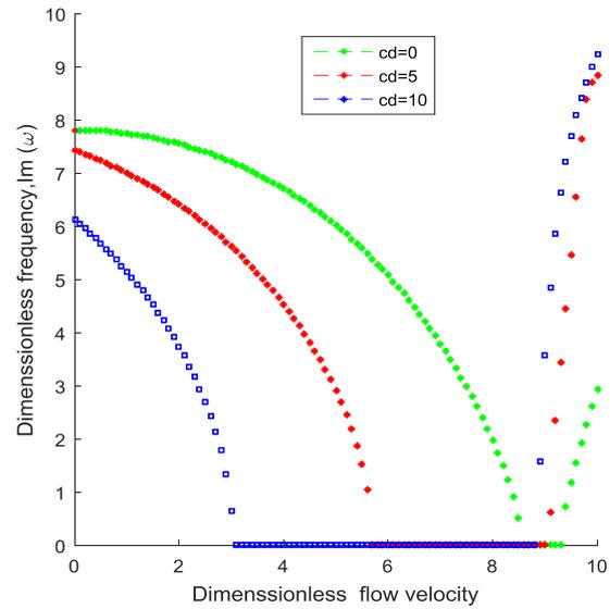
Fig. 7: Effect of damping foundation parameter on first natural frequency for (C-F) FG pipe with different flow velocity.
