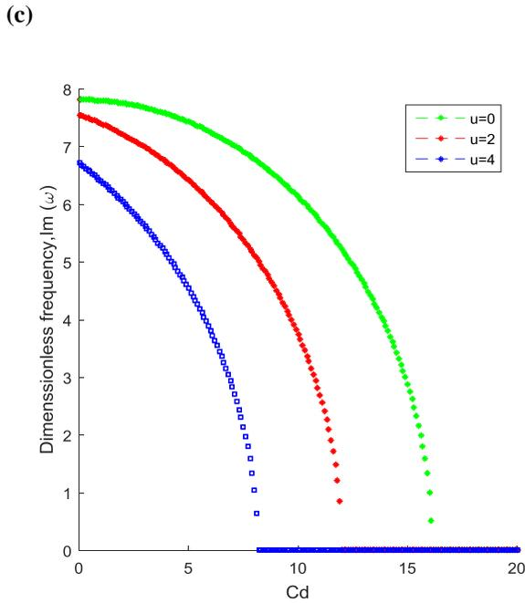
Fig. 6: Effect of visco-elastic foundation parameter on first natural frequency for (C-F) FG pipe with different flow velocity  $u$ , a) ( $K_s = 20, C_d = 10, k = 1$ ), b) ( $K_m = 50, C_d = 10, k = 1$ ), and c) ( $K_m = 50, K_s = 20, k = 1$ )
