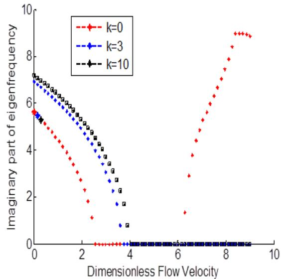
**Fig. 4:** The first mode of (C-F) FG pipe lying on visco-elastic foundation against fluid velocity  $u$  for different values of gradient index  $k$  ( $K_m = 50, K_s = 10, C_d = 10$ ).
