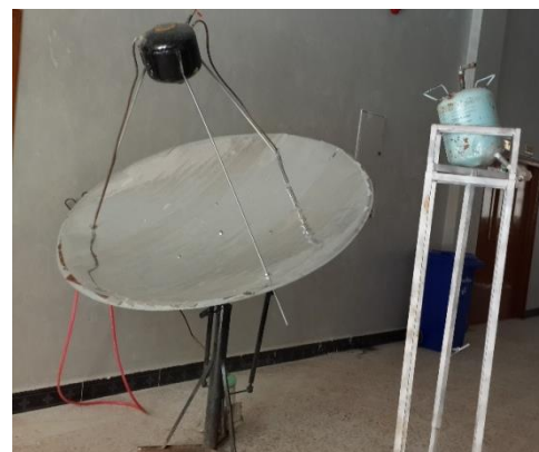
Fig. 2 Rig2 demonstration of parabolic concentrated dish
