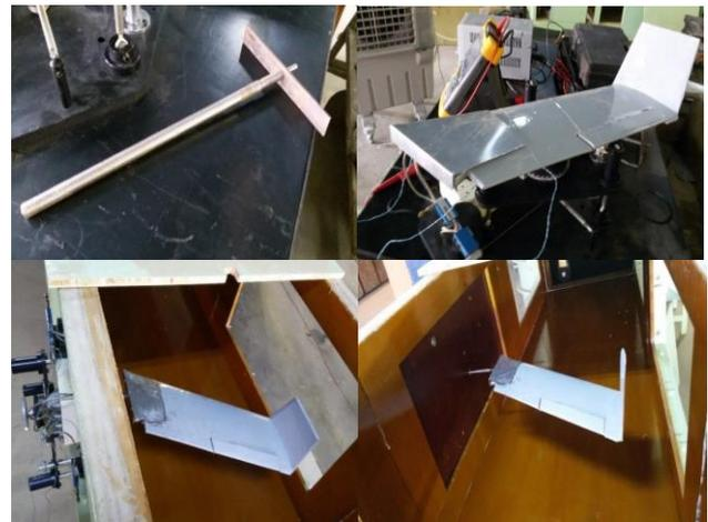
**Fig.3** Method of installing the test model inside wind tunnel.
