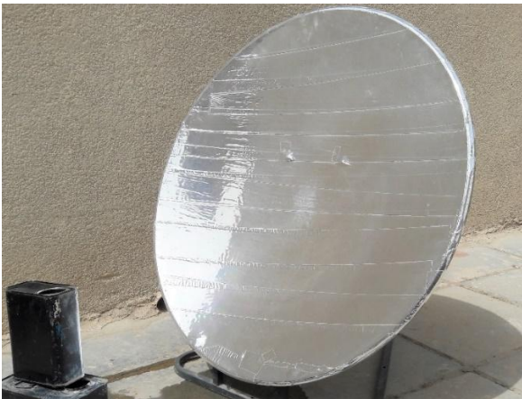
Fig.4 Experiments when using a parabolic solar concentrator with an Al- foil reflector.
