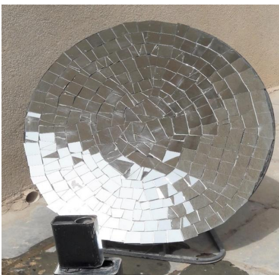
Fig.5 Experiments when using a parabolic solar concentrator with pieces of mirror reflector.
