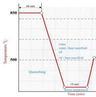
Fig. 5. Diagram illustration cycle of heat treatment used in this work.
