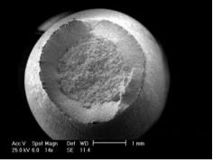
Fig. 18. fracture surface at CK35 steel after quenching at oil and nanofluid oil and tempering at 500°C.
