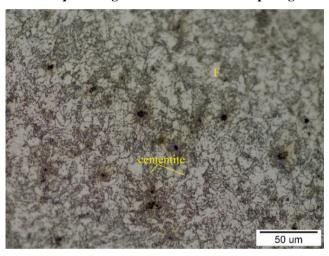
Fig. 11. Optical micrograph of microstructure of CK35 after quenching at oil and tempering.
