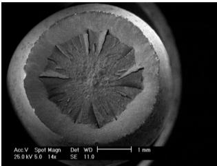
Fig. 12. Cup-cone geometry of ductile fracture at CK35 steel after quenching and tempering.
