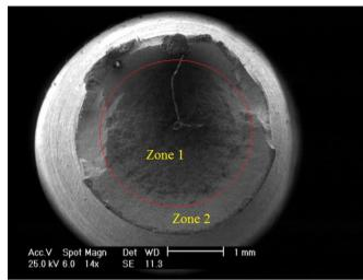
Fig. 16: fracture surface at CK35 steel after quenching at water and tempering at 500°C.
