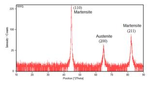
Fig. 7. X-ray diffraction profiles of CK53 after quenching at nanofluid water and tempering.
