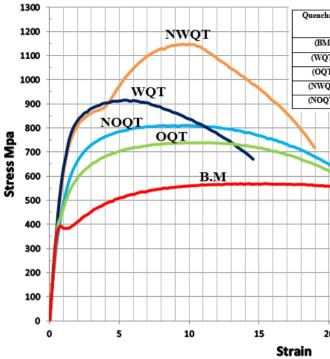
Fig. 6. Engineering stress-strain curves for CK35 at different quenching media.
