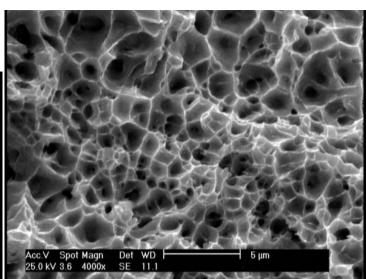
Fig. 17: Dimples (microvoid) on the fracture surface of CK35 steel tensile test piece.
