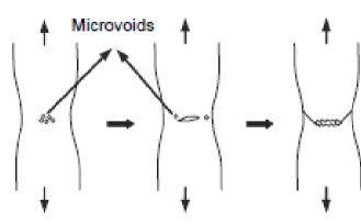
Fig. 13. Graphic illustration of the cup-cone geometry creation through the ductile fracture process [21].
