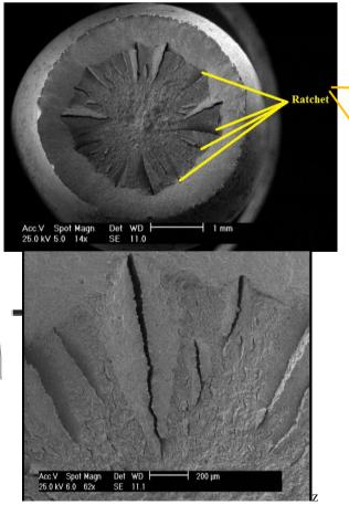
Fig. 15: Ratcheting marks observed during tensile of CK35 steel ruptured by tensile test.
