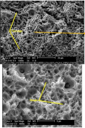
Fig. 14. Dimples (microvoid) in the fracture surface of CK35 tensile test piece.
