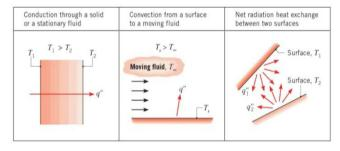
Fig. 3. Conduction, convection and radiation heat transfer modes [15].
