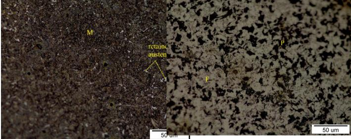
Fig. 8. Optical micrograph of microstructure of CK35 after quenching at nanofluid water and tempering.
