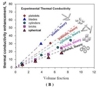
Fig. 2. A: Thermal conductivity (Keff/kf) enhancement as a function of volume fraction of particles [10]. B: Influence of the particle shape in the Thermal conductivity (Keff/kf) enhancement of Al<sub>2</sub>O<sub>3</sub>
