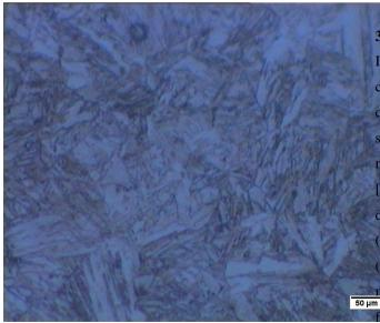
Fig. 9. Optical micrograph of microstructure of CK35 after quenching at water and tempering.
