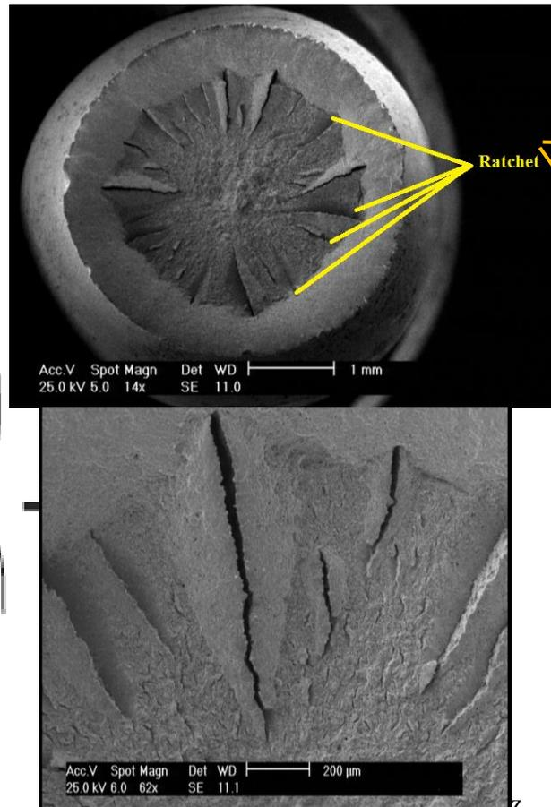
**Fig. 15: Ratcheting marks observed during tensile of CK35 steel ruptured by tensile test.**
