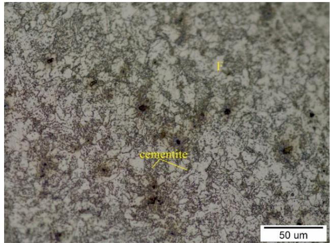
Fig. 11. Optical micrograph of microstructure of CK35 after quenching at oil and tempering.
