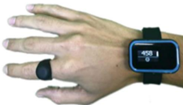
Fig.13 The Manometer consists of a ring with a permanent magnet and a sensing wrist. [28].
