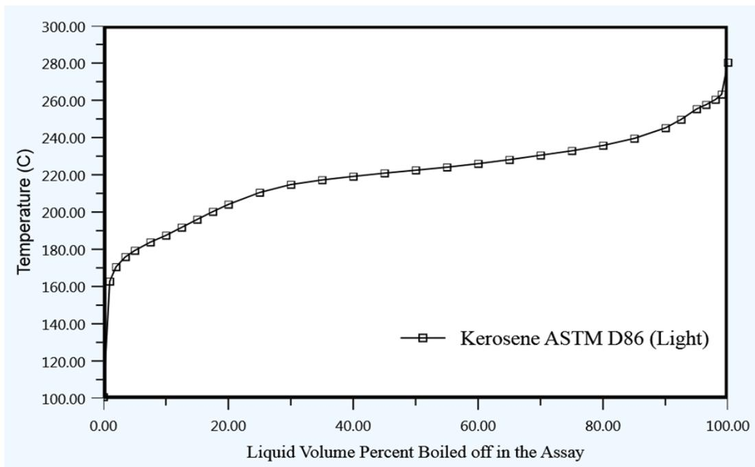
Figure 4: Simulated ASTM D86 curves of Kerosene.
