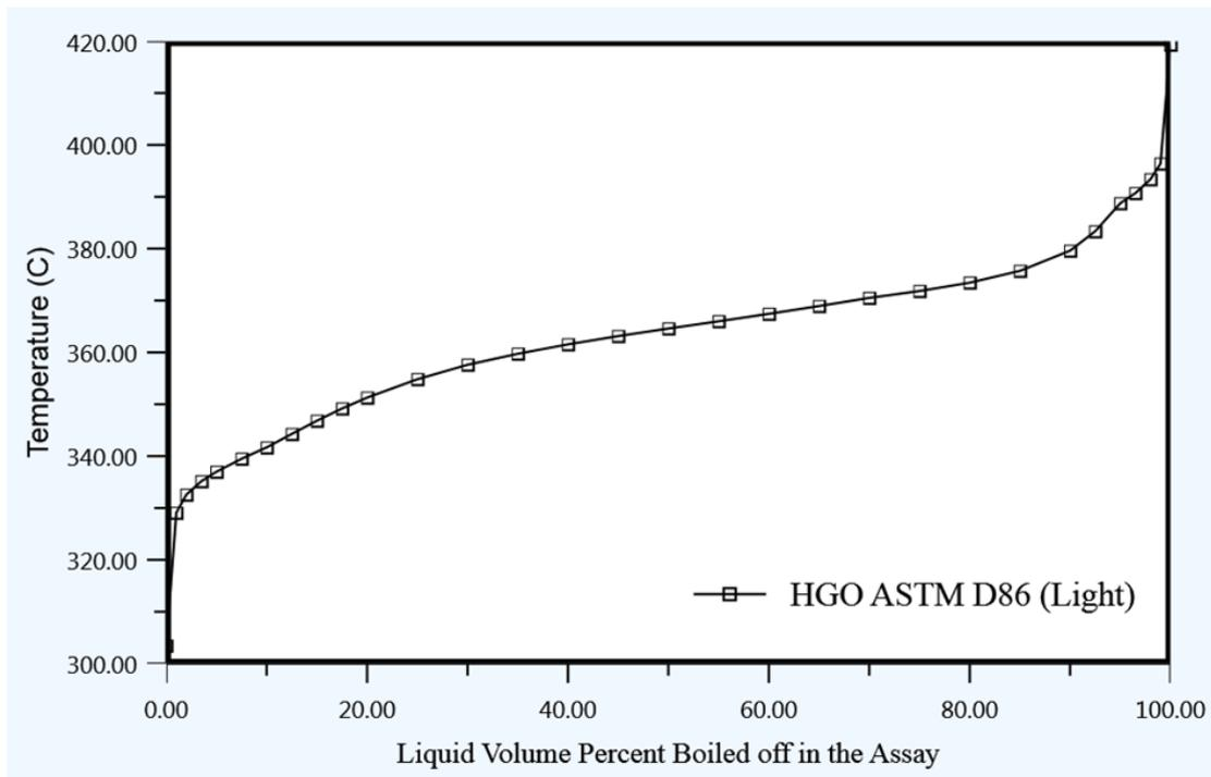
Figure 6: Simulated ASTM D86 curves of HGO.
