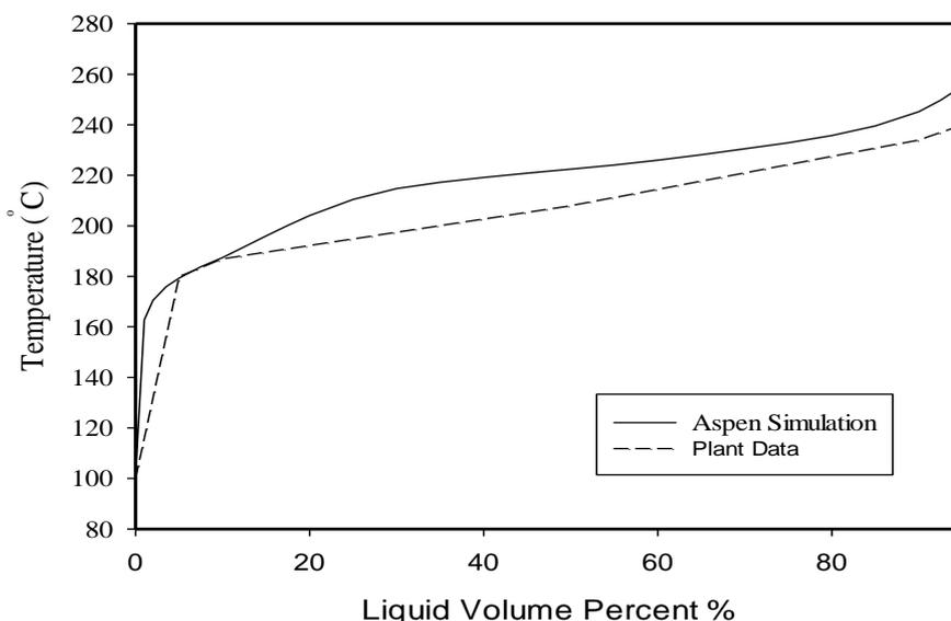
Figure 7: Simulated and plant data ASTM D86 curves of Kerosene.
