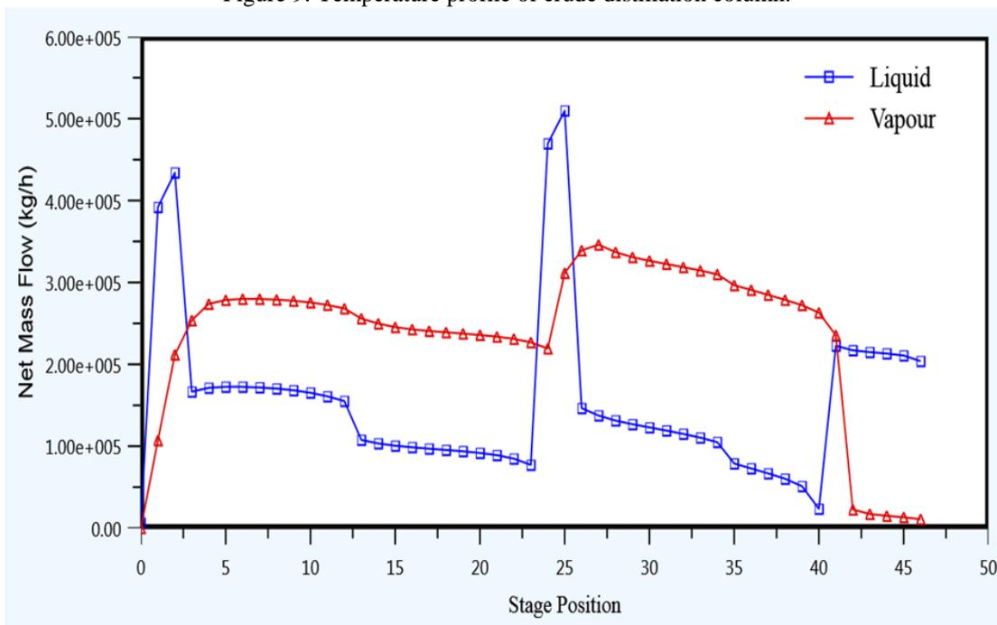
Figure 10: simulated mass flow rates for vapor and liquid phases within the column.
