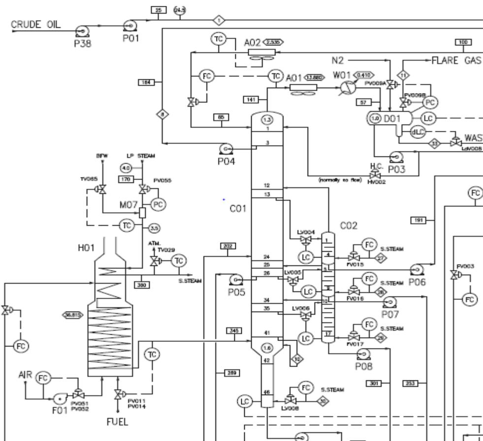
Figure 2: Crude distillation unit in Basrah refinery.
