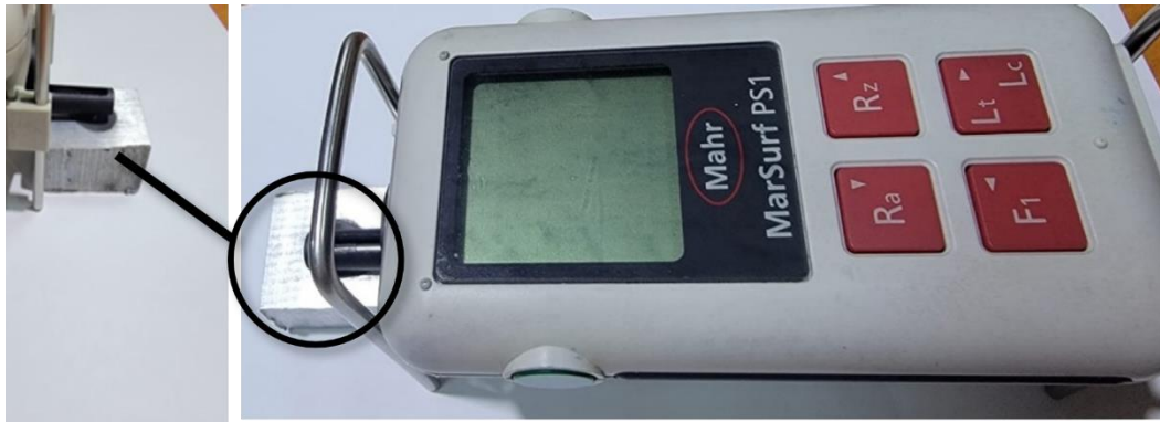
Figure 4: Mahr Pocket Surf PS1 Portable Surface Roughness Tester.
