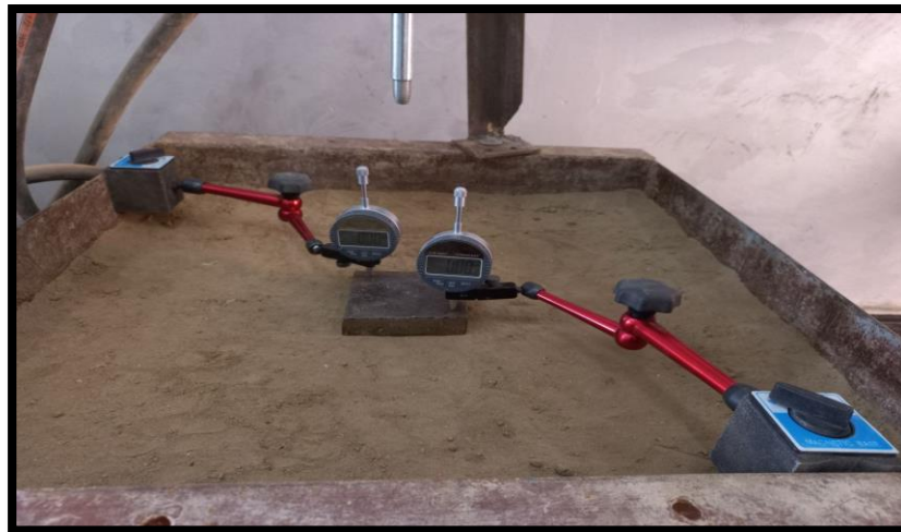
Figure 3: Dial gage and magnetic stands using in work
