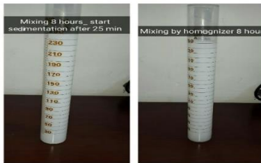
c- Sedimentation of mixture which mixing by homogenizer for 8 hours
