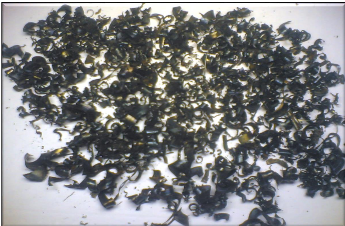
Fig. (1) Waste-iron produced from milling process
