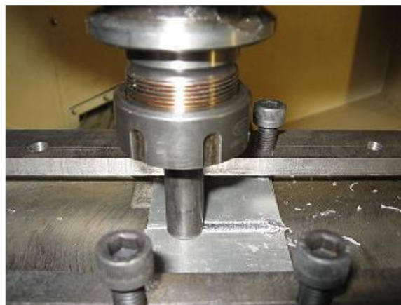
Figure (2) Friction stir welding process
