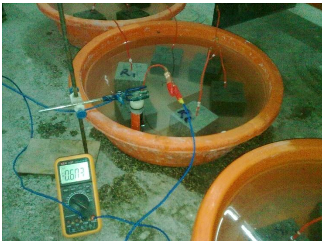
Figure1: corrosion potential measurement
