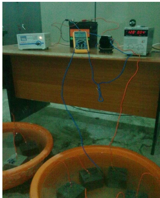
Figure 2: Electrical connection for applying a +12 V fixed anodic potential to accelerate the corrosion
