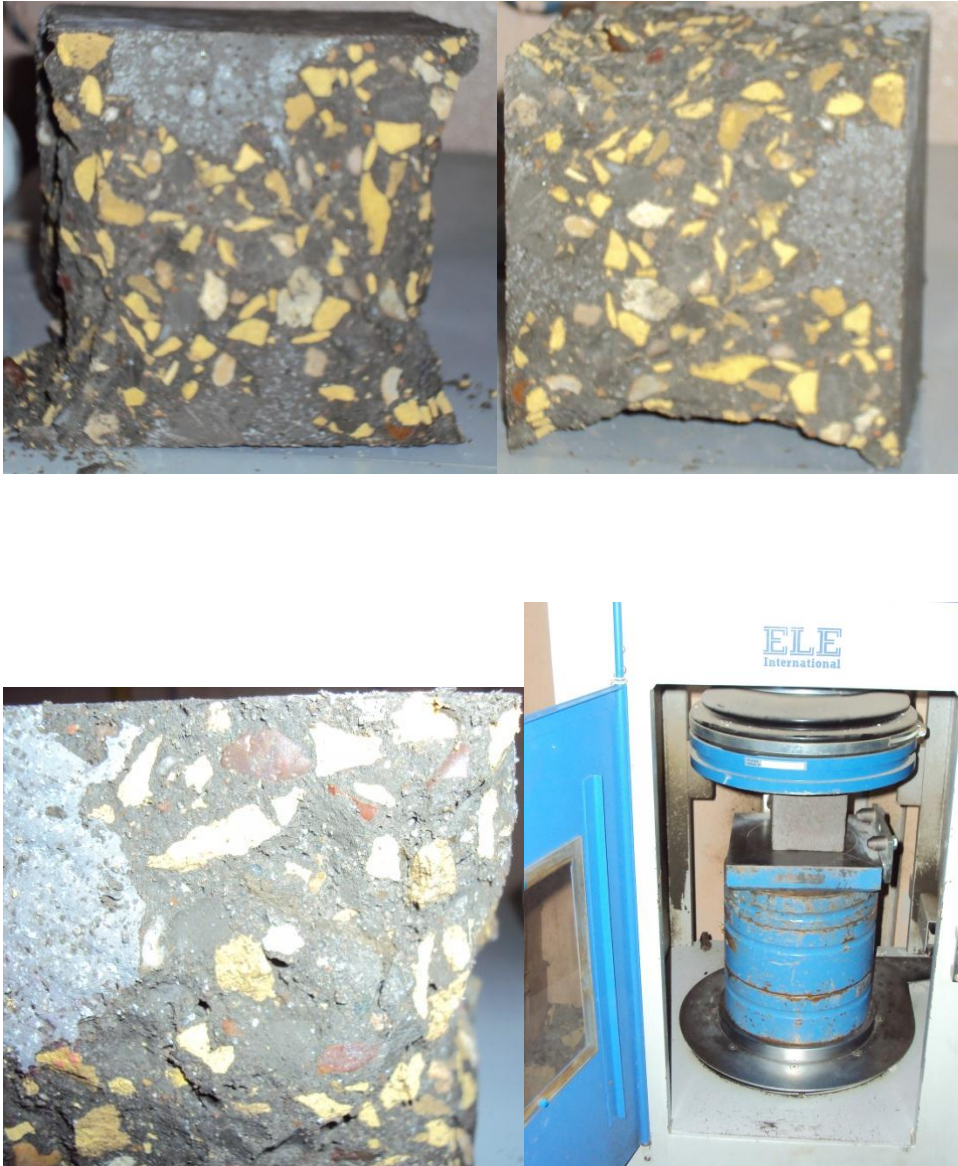
Figure (7) shows cubes under test and failure samples
