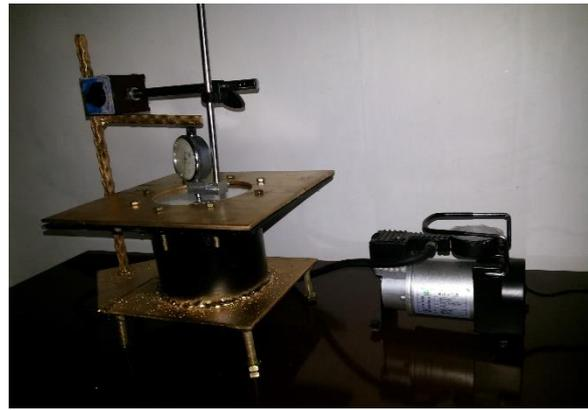
Fig. ( 3 ). Device made for testing clamped at the edges of circular plate
