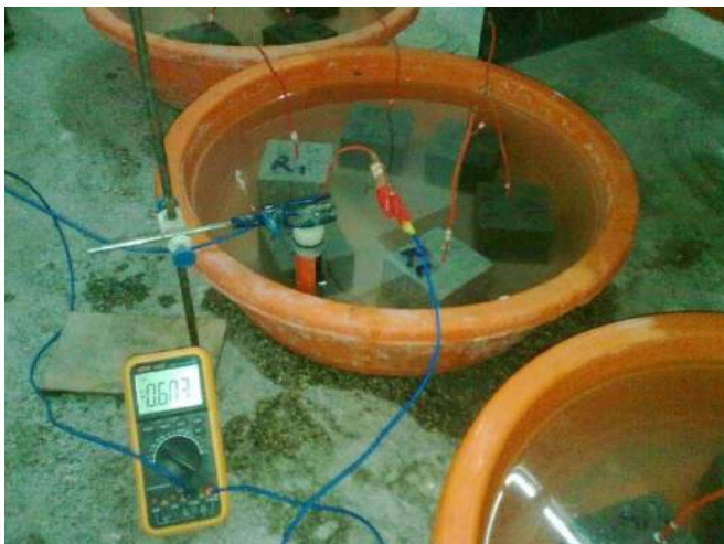
Figure1: corrosion potential measurement
