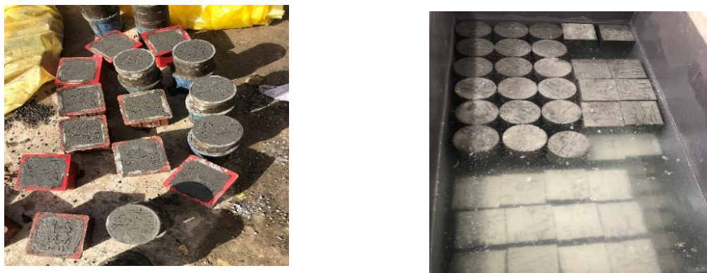
Figure 2: The casting and curing processes of samples
