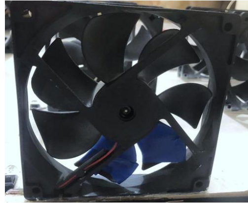
Figure 2: Defected fan with insulation tape on two blades
