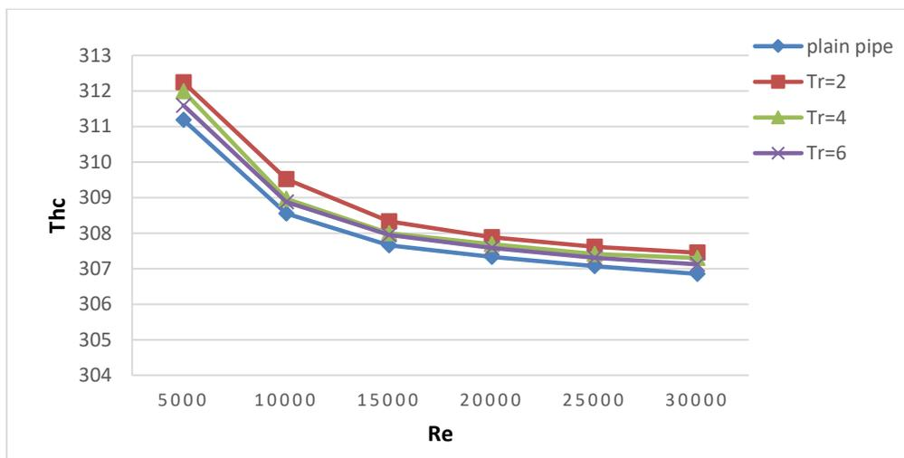
Figure 6: Variation of cold fluid outlet temperature with Re for DTTEH
