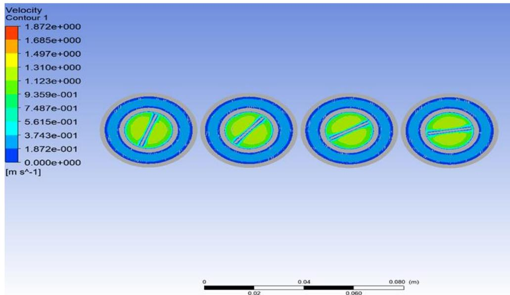
Figure 11: Cross-section velocity contour at ( $x=0.2$ ,  $x=0.4$ ,  $x=0.6$ ,  $x=0.8$ ) m for DTTHE
