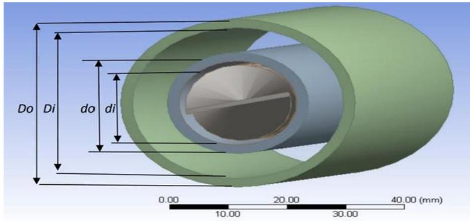
(a) Cross-section of for double pipe heat exchanger with the twisted tape
