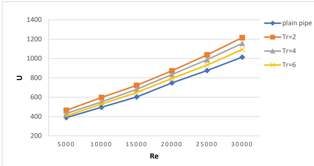
Figure 9: Variation of the coefficient of overall heat transfer versus Reynolds number
