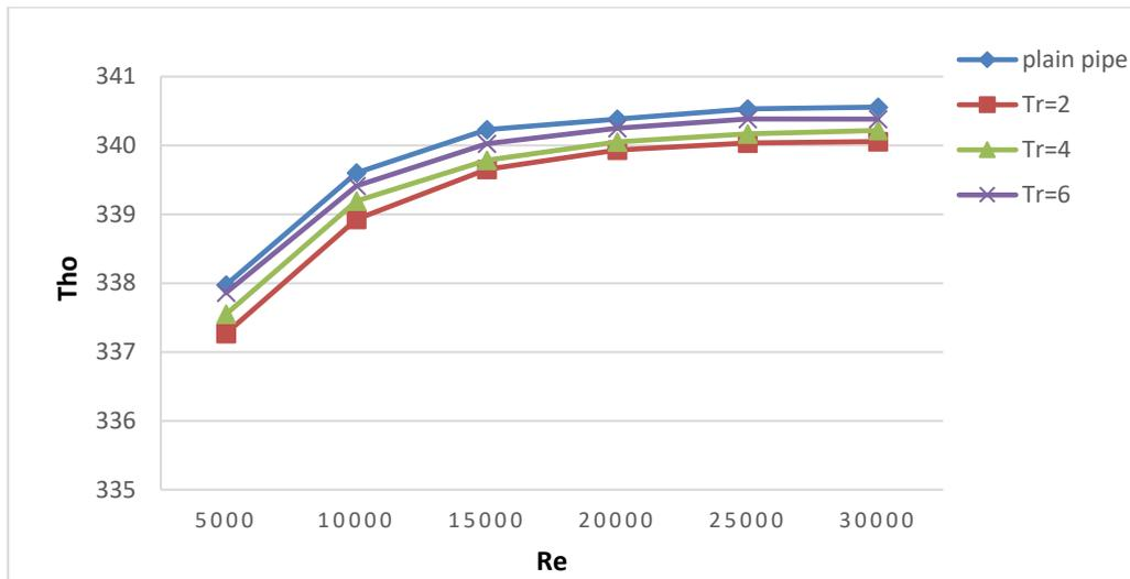
Figure 5: Difference of the hot fluid outlet temperature with Re for DTTEH
