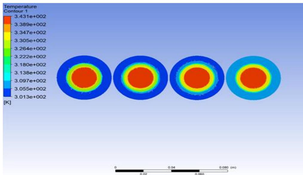
Figure 10: Cross-section temperature contours of the hot and cold fluid at (x=0.2, x=0.4, x=0.6, x=0.8)m for DTTHE at Re (30000)
