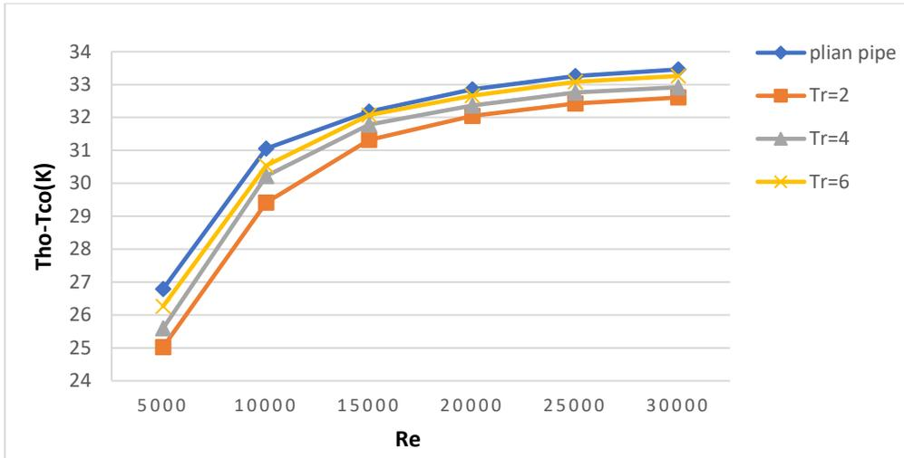
Figure 7: The difference between hot and cold fluid outlet Temperature with Re for DTTHE
