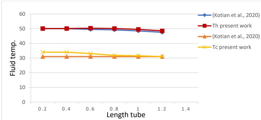
Figure 3: Validation of hot and cold liquid temperature between the present results and the results of (Kotian et al., 2020) published
