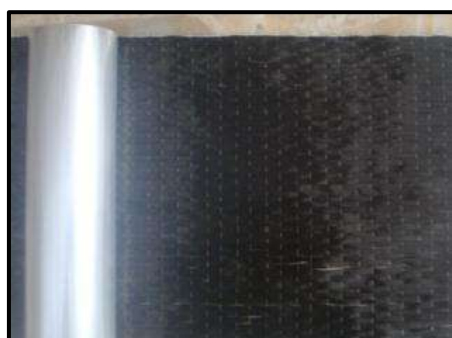
Plate(2) Aluminum tube and CFRP before retrofitting
