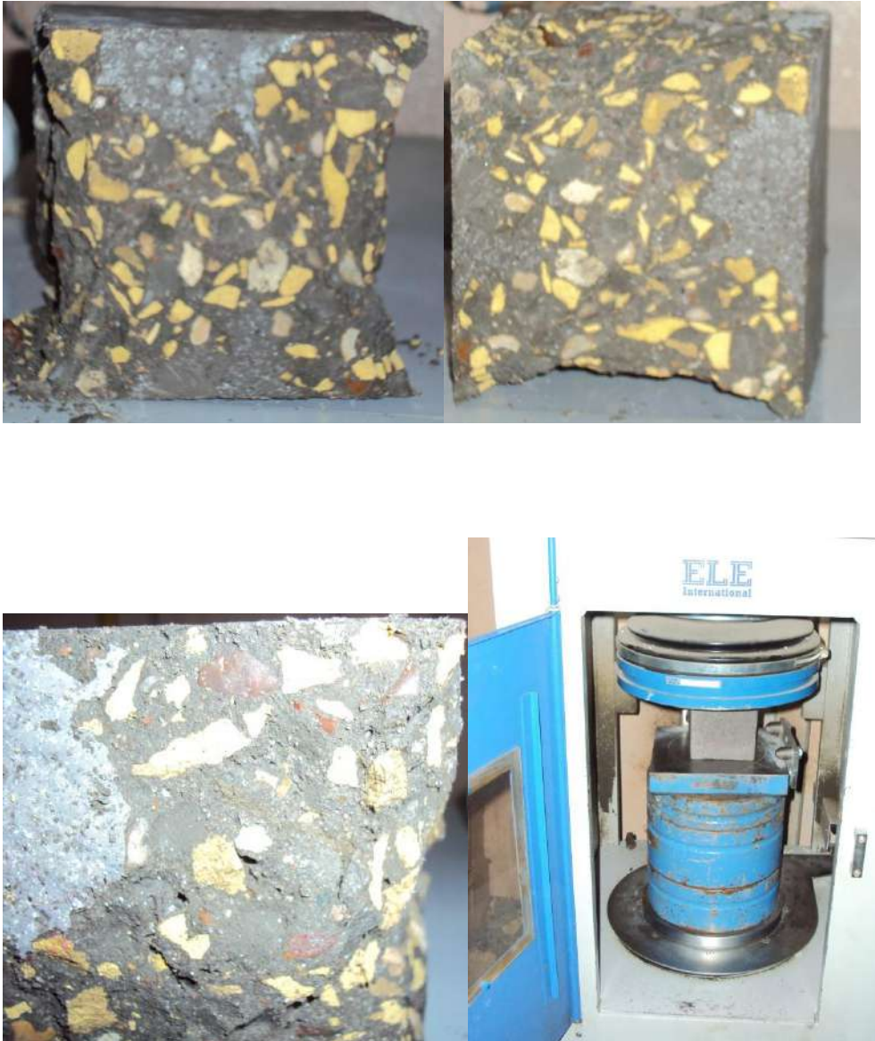
Figure (7) shows cubes under test and failure samples
