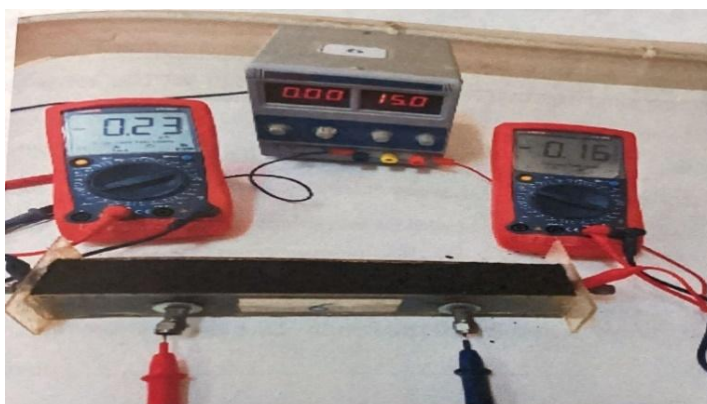
Figure 9: Electrical setup for a four-electrode resistivity soil testing box (N. K. Al-Obaigy et al., 2020)
