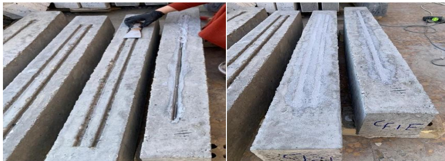
Figure 6: Strengthened beams using NSM with epoxy
