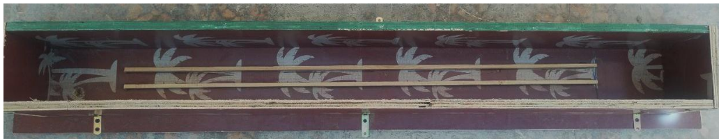
Figure 4: Formation groove in the wooden mold
