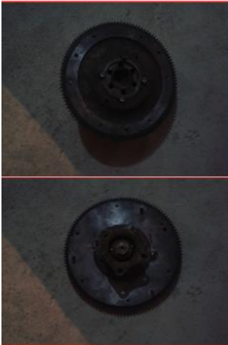
Fig.1 Gears used for azimuth movement
