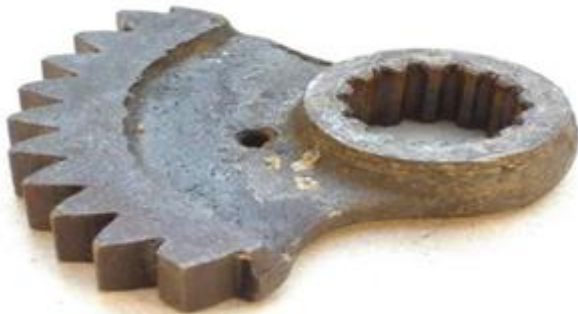
Fig. (2) Gear used for elevation movement
